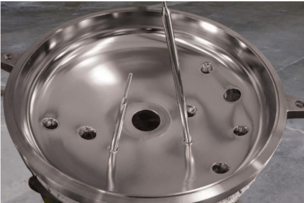
*Process tanks in the pharmaceutical industry are electropolished to meet the highest hygiene requirement. Photo: Centro Inox, Milan (I)*
